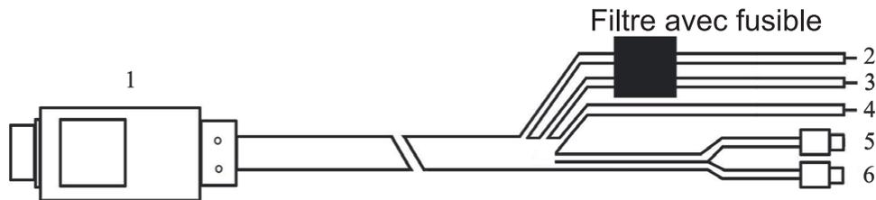
**NOTE : SI VOUS CONNECTEZ CORRECTEMENT LE FIL VERT (CAPTEUR DE MARCHÉ ARRIÈRE) AU PÔLE POSITIF DU FEU DE MARCHÉ ARRIÈRE, DÈS QUE LA MARCHÉ ARRIÈRE EST ENCLANCHÉE, LE MONITEUR AFFICHERA L'ENTRÉE V2 MÊME S'IL EST ÉTEINT.**
